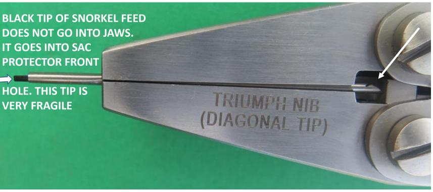
DIAGONALLY CUT SIDE OF SNORKEL IS SHOWN HERE, SEATED ON ITS STOP. THIS END OF SNORKEL IS ALSO VERY FRAGILE AND MUST BE *GENTLY*FITTED INTO ITS GROOVE AND GENTLY SEATED ONTO ITS STOP BEFORE SQUEEZING HANDLES AND PUSHING SNORKEL INTO PLASTIC PLUG ON SAC PROTECTOR FRONT.
