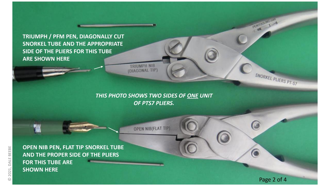
The diagonally cut snorkel tip from pens with Triumph or PFM nibs goes INTO the slot on the side marked "TRIUMPH NIB (DIAGONAL TIP)".
